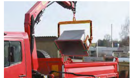
Tipping the grit out onto a truck platform (shown with 700 L the grit bin)
