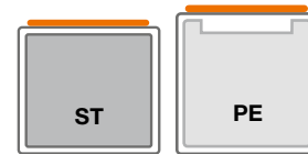
DT-Mobil PRO Outer container in steel, inner container in steel or PE
