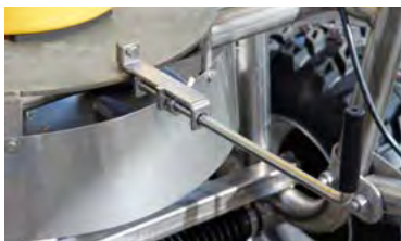
Spreading quantity control
