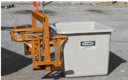
Engaging the loading frame from the side after removal of the removable lid (shown with 700 L grit bin)
