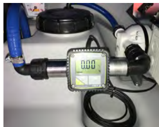
Meter FMT 3 with pulse output
