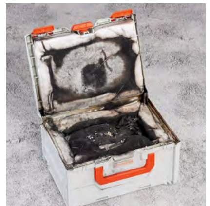
Successful fire test: the CEMO fire prevention box withstands the flames.
